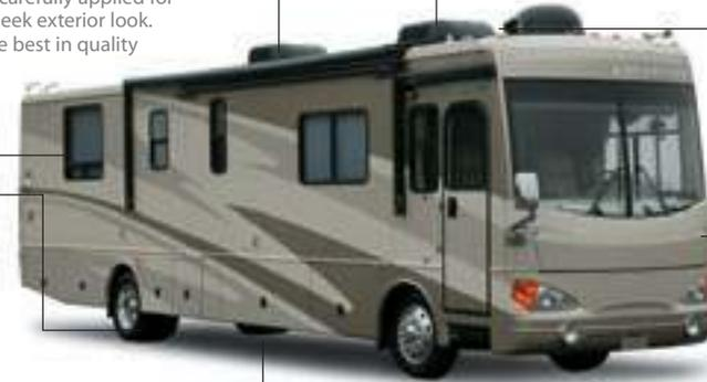
**STORAGE COMPARTMENTS** are lighted and include single paddle metal latches, gas-lift strut supports, stainless-steel hinges and insulated aluminum doors.
