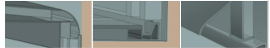
Inter-locking Ceiling-to-Sidewall Connection
