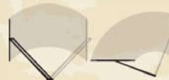
Pantographic Windshield Wipers (left) such as those installed on Sea Breeze motorhomes clean a wider swath of windshield than typical radial windshield wipers (right) of similar blade length.
