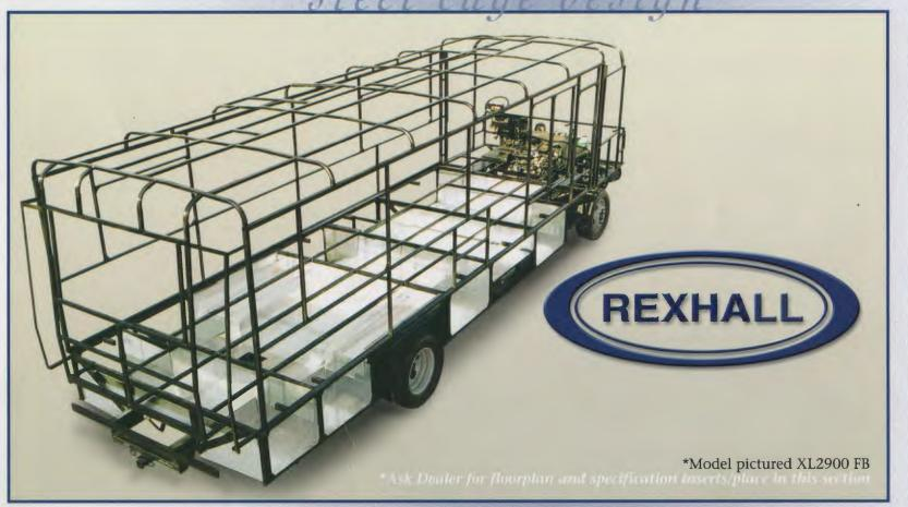
by exposing the steel in our 2" vacuum bonded sidewall, you can see the welded (not screwed) Uni-Body Steel Cage that makes the difference in strength, value and safety in a Rexhall motorhome.
