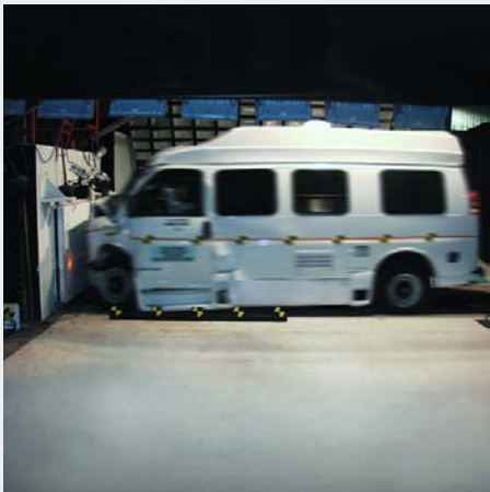
For frontal impact testing of the 190 Chevy, the test vehicle impacted a fixed barrier at 30-mph (48 km/h). Again our test vehicle did not leak any fuel.
