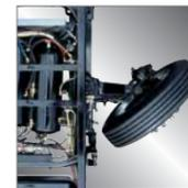
Sharp, 55 degree wheel cut enables superior maneuvering in tight spaces.
