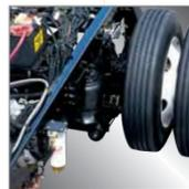
Standard full air ride suspension provides a comfortable ride with reduced body roll.
