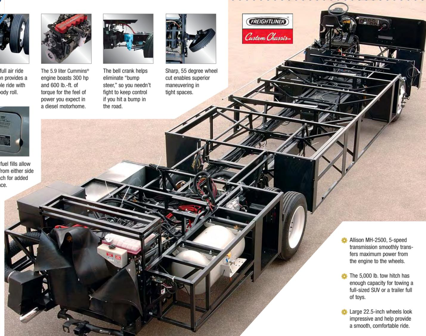
✿ Allison MH-2500, 5-speed transmission smoothly transfers maximum power from the engine to the wheels.
