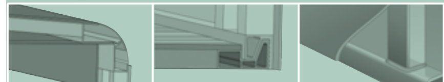
Inter-locking Ceiling-to-Sidewall Connection
