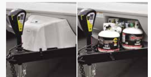
Optional Tri-Five Propane Tanks allow for extended stays while standard aerodynamic cover looks stylish and keeps tanks protected and out of site. - N/A 1475 & 1575
