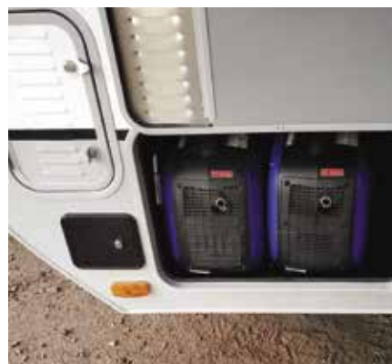
Portable generator storage compartment with tie down straps, accommodates Honda 2100 and similar sized portable generators. - N/A 1475, 1575 & 2465.
